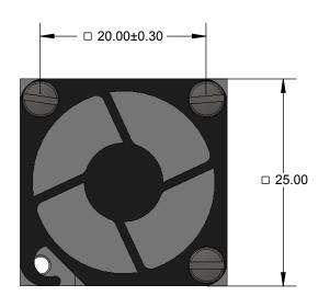
This heat sink compression screw is compatible with all Ironwood low profile swivel lid sockets for IC sizes <10mm and socket lids with M6 threads.
