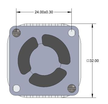
This heat sink compression screw is compatible with all Ironwood low profile swivel lid sockets for IC sizes >20mm to <30mm, and socket lids with M10 threads.
