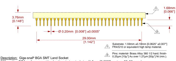
900 position BGA surface mount land pattern to terminal pins (1.0mm [0.039"] centers, 30x30 array)
