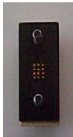
Fig. 2 Pin block with spring probe array
