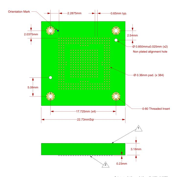
Substrate: 3.18mm  $\pm 0.18$ mm [0.125"  $\pm 0.007$ "] FR4/G10 or equivalent high temp material. 17µm [1/2 oz.] Cu clad.
