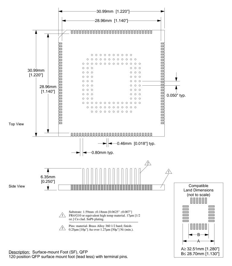
Tolerances: diameters ±0.03mm [±0.001"], PCB perimeters ±0.13mm [±0.005"], PCB thicknesses ±0.18mm [±0.007"], pitches (from true position) ±0.08mm [±0.003"], all other tolerances ±0.13mm [±0.005"] unless stated otherwise. Materials and specifications are subject to change without notice.
