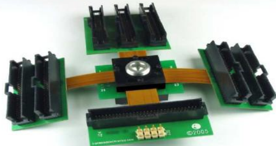
0.5mm pitch 21x21 array 289 position BGA solder balls to AMP 104068 connectors using rigid flex PCB with socket fixture
