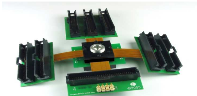
0.5mm pitch 21x21 array 289 position BGA solder balls to AMP 104068 connectors using rigid flex PCB with socket fixture
