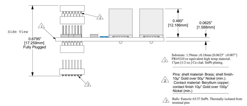
Description: LA adaptor for TEKTRONIX TLA700 series Logic Analyzer
