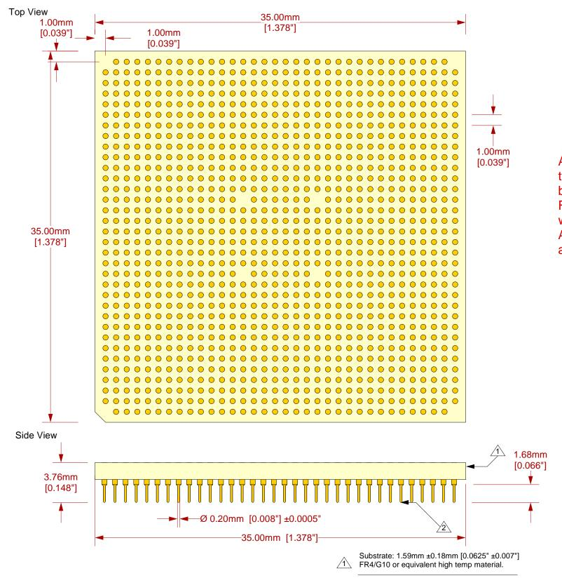
Pins: material- Brass Alloy 360 1/2 hard; finish-0.25μm [10μ"] Au over 1.27μm [50μ"] Ni (min.).
