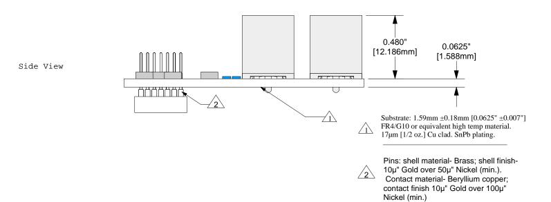
Description: Probe Board for TEKTRONIX TLA700 series Logic Analyzer
