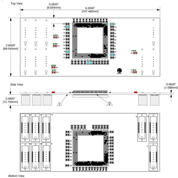
Substrate: 1.59mm ±0.18mm [0.0625" ±0.007"] FR4/G10 or equivalent high temp material. 17µm [1/2 oz.] Cu clad.
