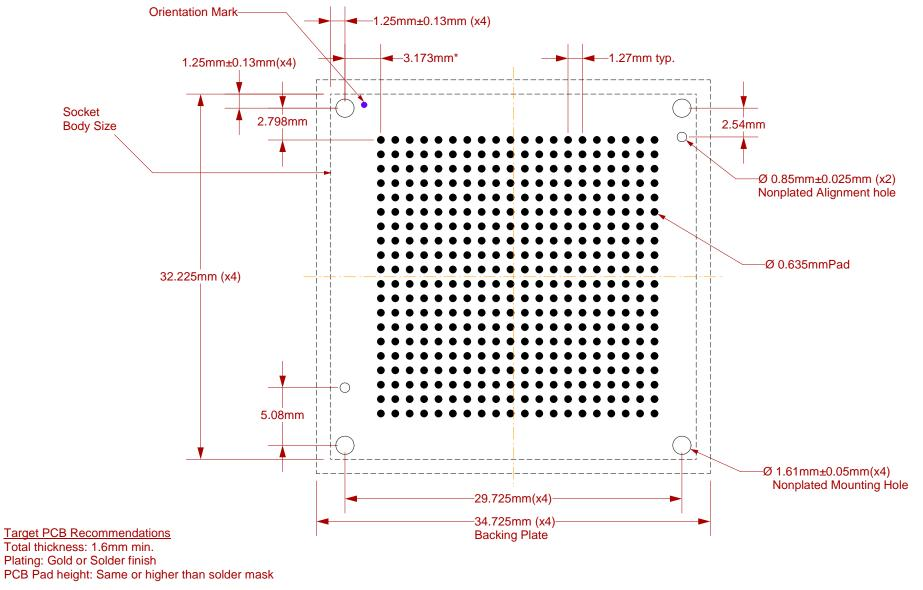
NOTE: Steel backing plate may be required based on end user's application
