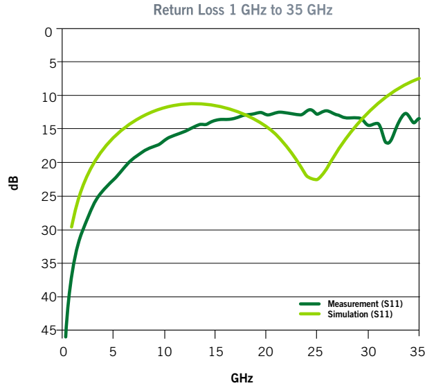
Figure 5. GSG P2A Return Loss comparison, 0.8 mm pitch
