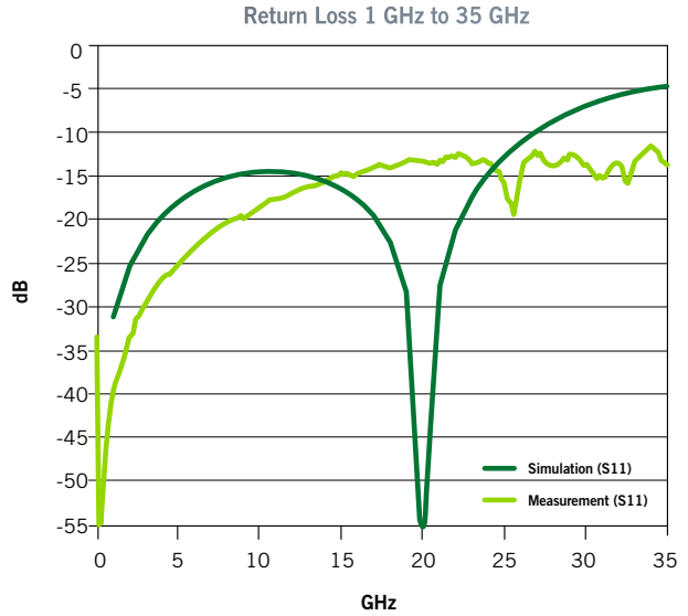
Figure 5. GSG P2A Return Loss comparison, 0.8 mm pitch
