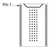
Orient Pin 1 of foot with respect to pin one of SOIC
