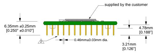
Substrate: 1.59mm ±0.18mm [0.0625" ±0.007"] FR4/G10 or equivalent high temp material. 17µm [1/2 oz.] Cu clad. SnPb plating.
