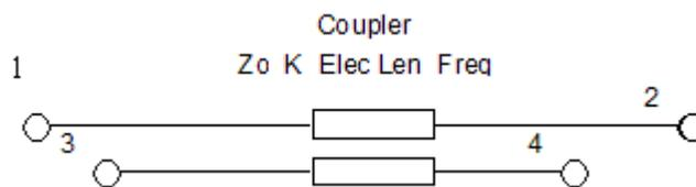
Figure 36 Transmission line equivalent circuit for crosstalk
