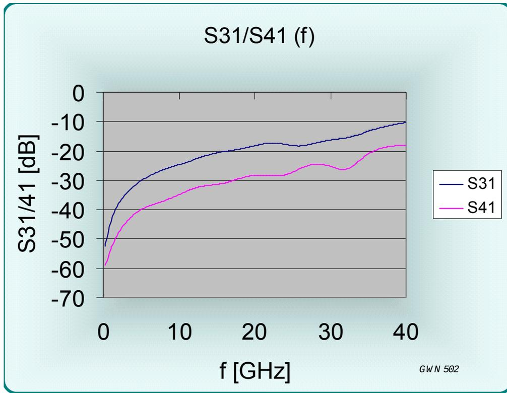
Figure 27 Crosstalk as a function of frequency
