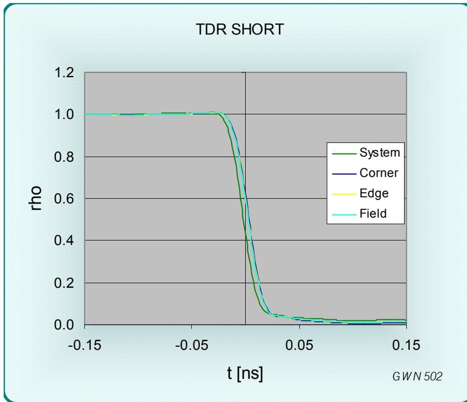
Figure 6 TDR signal from a SHORT circuited GTP contact
