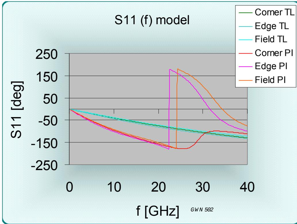
Figure 32 S11 phase (f) for open circuited case
