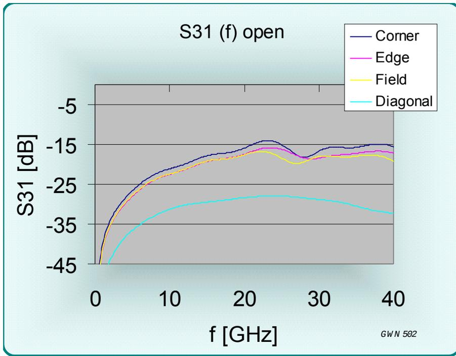
Figure 28 Open circuit crosstalk from port 1 to port 3
