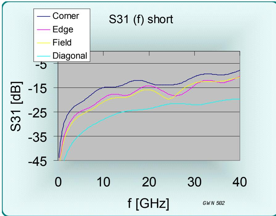
Figure 29 Short circuit crosstalk from port 1 to port 3
