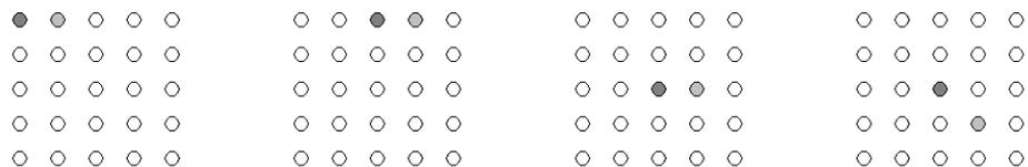
The second pin (light grey) is the second signal pin for G -S-S-G testing. Mutual parameters are also determined for the diagonal case. Configurations are referred to as G-S-G and G-S-S-G although strictly speaking this is not true. Signal pins are completely surrounded by ground pins since behavior would be very similar if they were connected to 50 Ohm driven pins as is the case in typical BGA environments.
