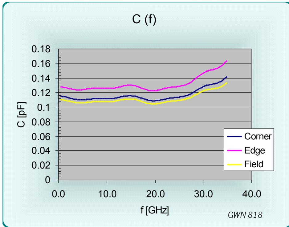
Figure 11 C(f) for the open circuited signal pin
