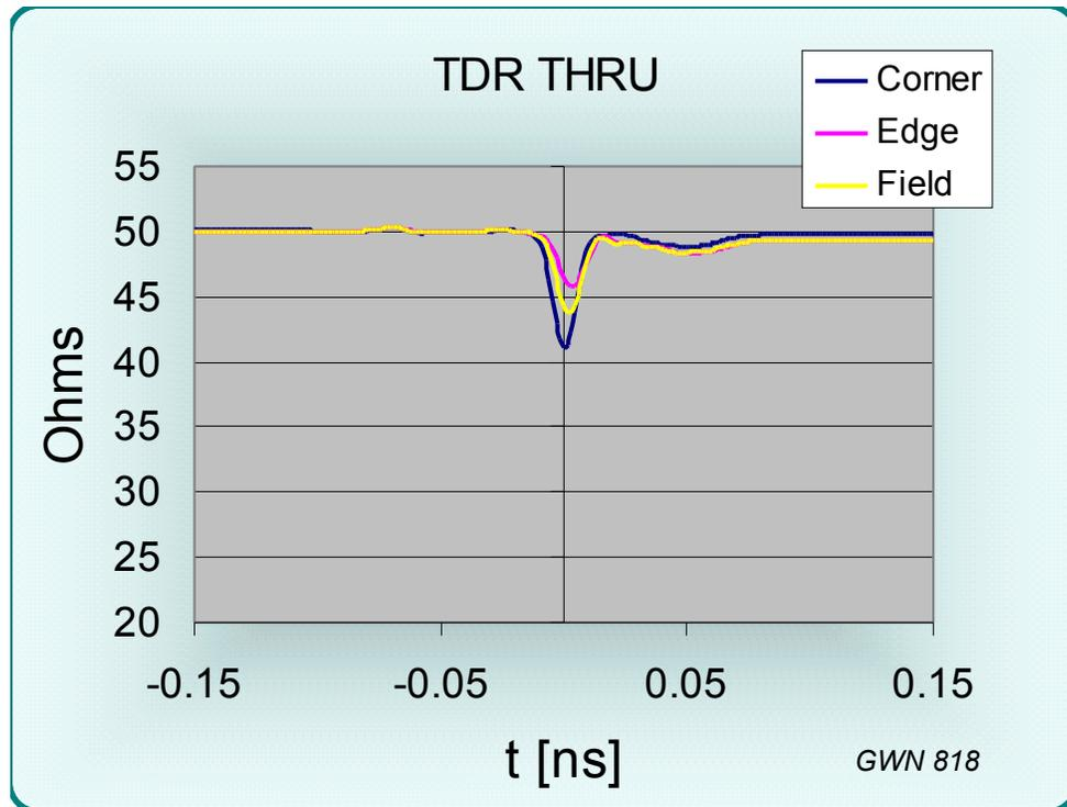
Figure 7 TDR measurement into a 50 Ohm probe
