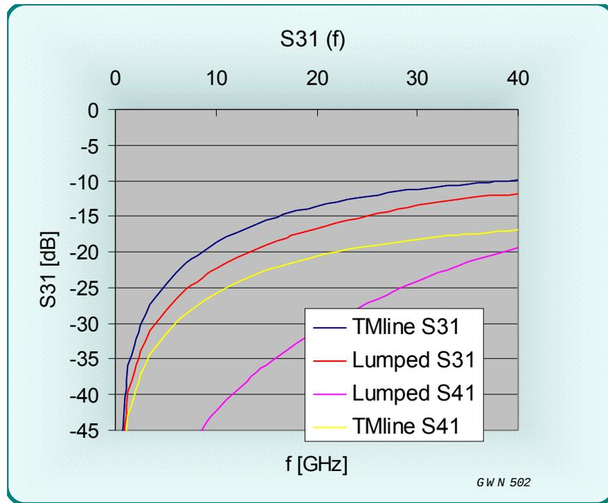
Figure 37 Crosstalk S31 and S41 [dB] as a function of frequency
