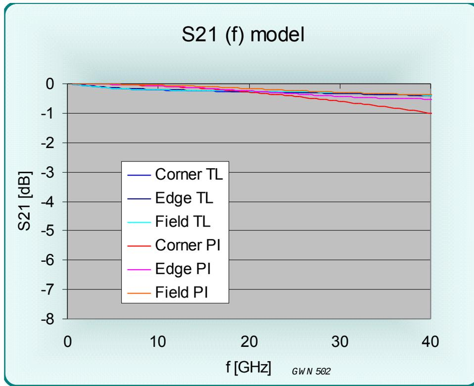
Figure 34 Insertion loss as a function of frequency
