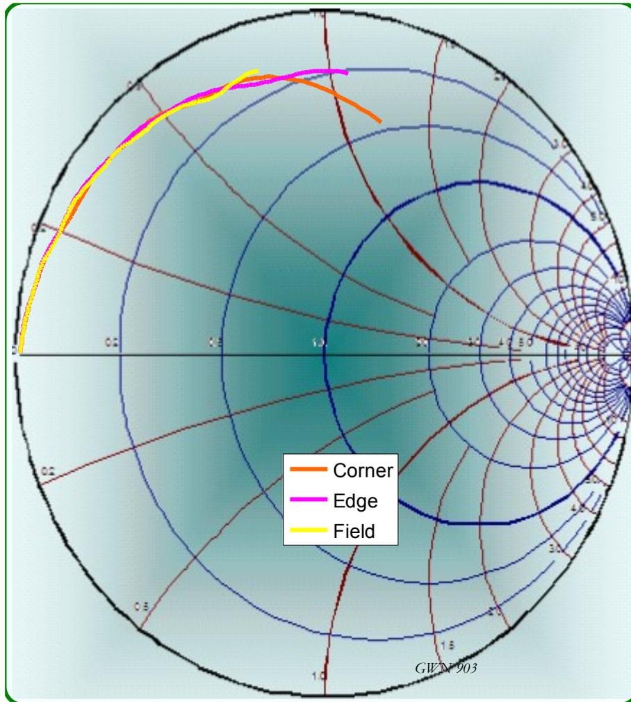
Figure 16 Short circuit response in the Smith chart
