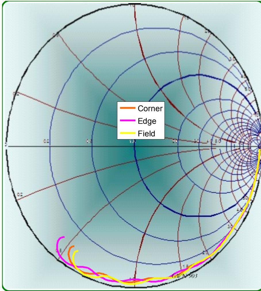
Figure 12 Reflections from the open circuited GTP contact
