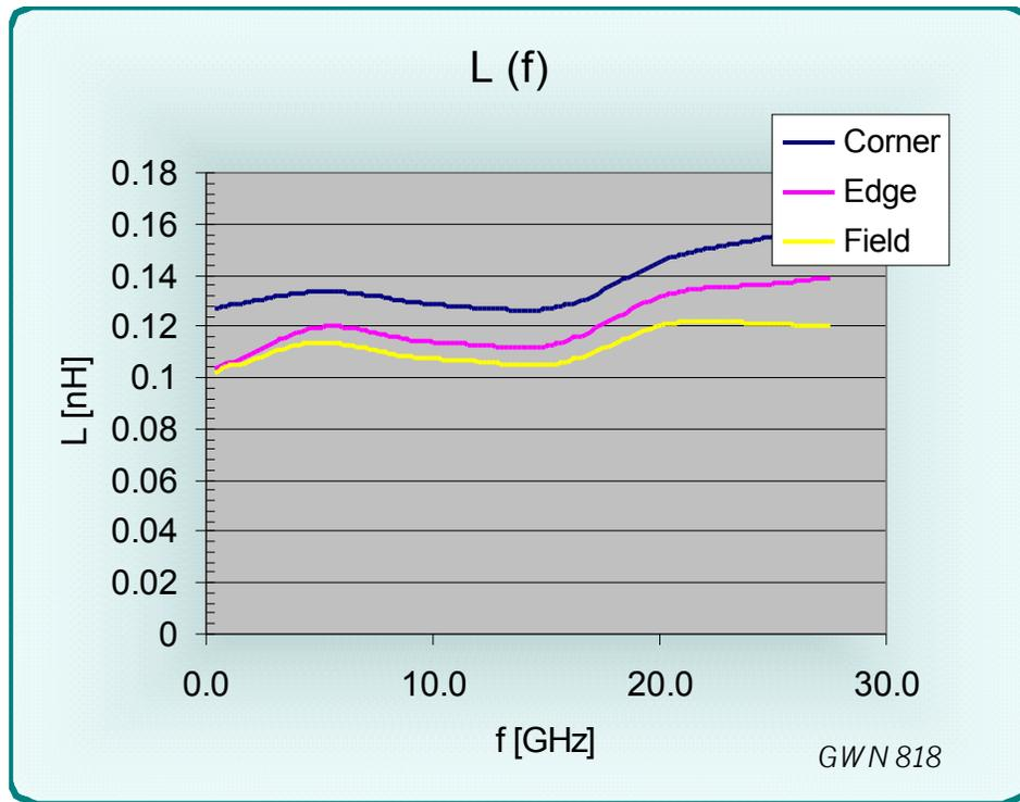
Figure 15 L(f) for the GTP contact
