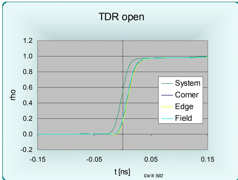
Figure 5 TDR signal from an OPEN circuited GTP contact
