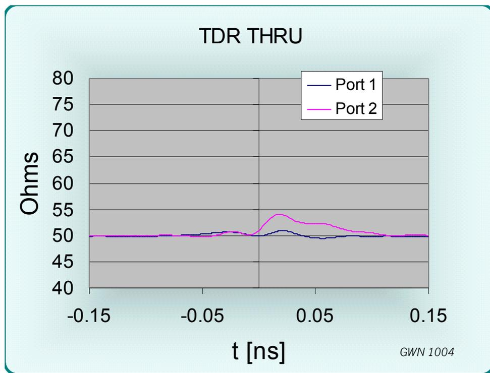
Figure 21 TDR through DUT into a terminated probe
