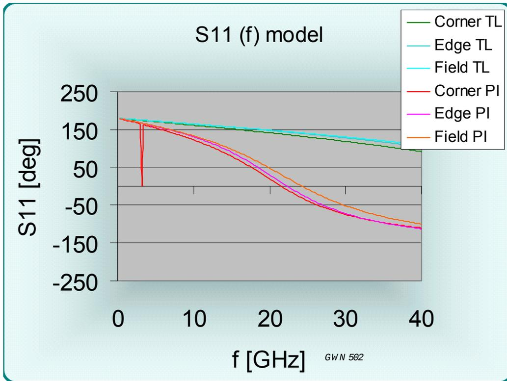
Figure 33 S11 phase response (short circuit)
