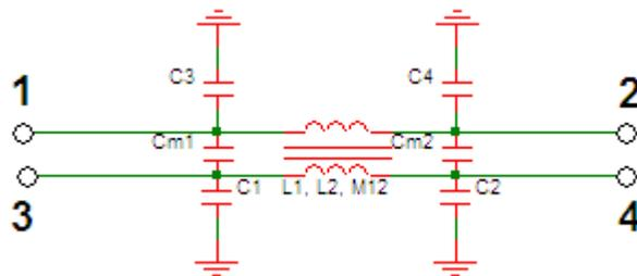
Figure 35 Equivalent circuit for G-S-S-G (mutual coupling)
