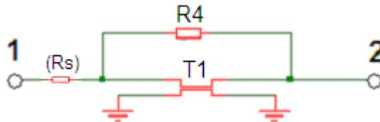
Figure 31 Transmission line model for the GTP contact
