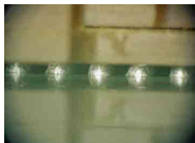
Test socket attached to the loadboard/PCB
