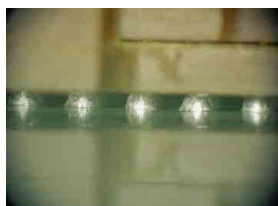
Test socket attached to the loadboard/PCB
