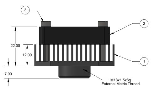
This heat sink compression screw is compatible with all Ironwood low profile swivel lid sockets for IC sizes 21mm to 29mm, and socket lids with M18 threads.
