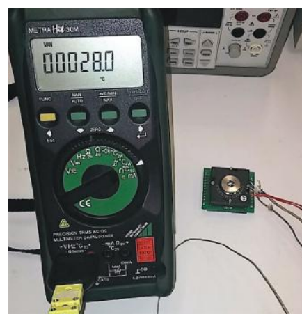
Figure 2: Experimental setup showing the compressed socket with heater element rod connected to a power supply and a thermocouple connected to a multimeter.
