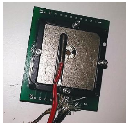
Figure 1: Experimental setup showing the heater element rod integrated into the socket compression plate.
