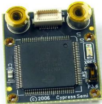
SoC module with high density connector
