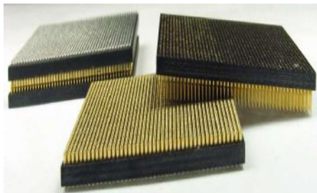
2000 pin count BGA adapter system plugged together IP, 1/23/2020
