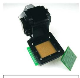
Figure 1: Spring Pin Socket
