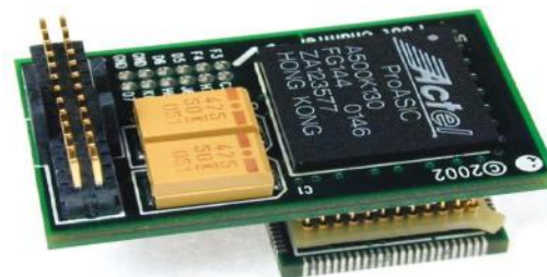
Daughter card module Interfaced to QFP footprint
