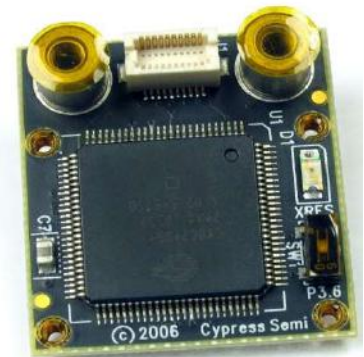
SoC module with high density connector
