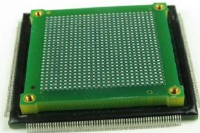
BGA device mounted to QFP footprint on mother board
