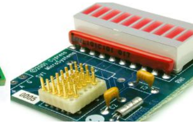
Dual technology (SMT & thru hole) assembly
