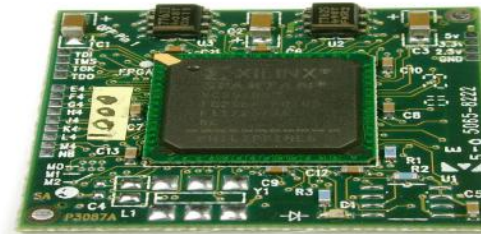
BGA device, discrete & voltage regulator
