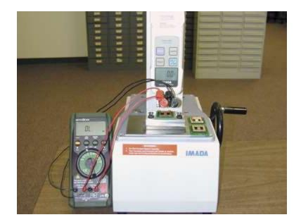
Figure 3: Insertion/Extraction test setup
