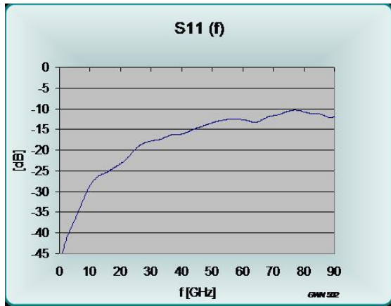
Figure 3: Return loss curve for elastomer socket that is graphed for frequency range up to 90GHz
