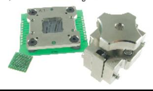
Solving both engineering and production needs, our adapters provide the capability to test and prototype in the laboratory as well as provide solutions that can provide IC package conversion that can keep a production line going when an IC becomes unavailable.
