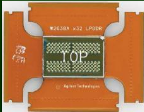
Four wing probe for DDR memory
