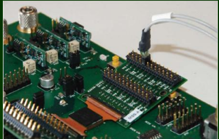
Two wing probe for DDR memory under test
