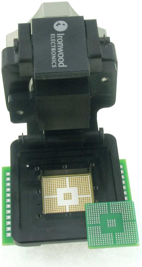
Figure 3 – 500K cycle, High endurance spring pin socket with removable clamshell lid
