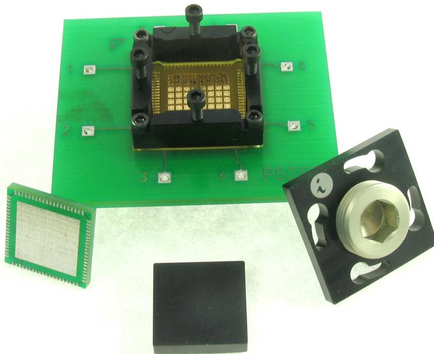
Figure 2 – 40GHz, Small footprint, Diamond particle interconnect socket
