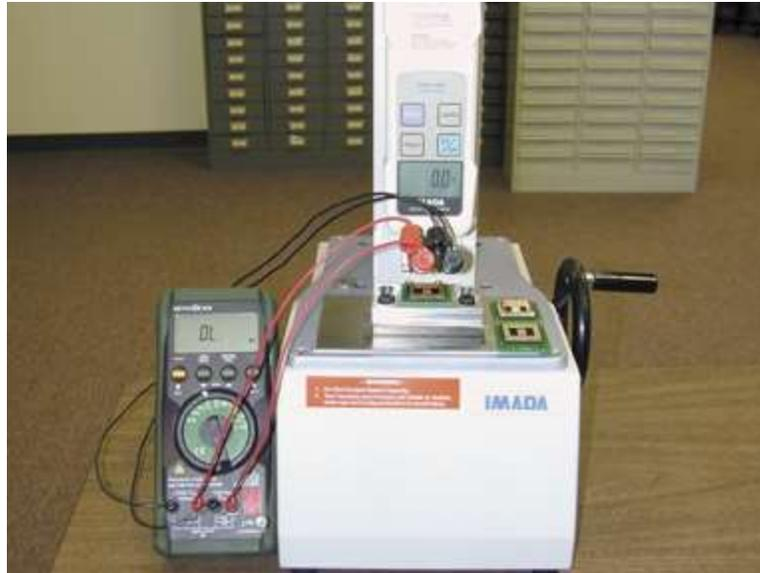
Figure 3: Insertion/Extraction test setup
