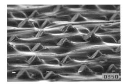
Protruded wire from elastomer
