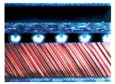
BGA compressed on Elastomer
