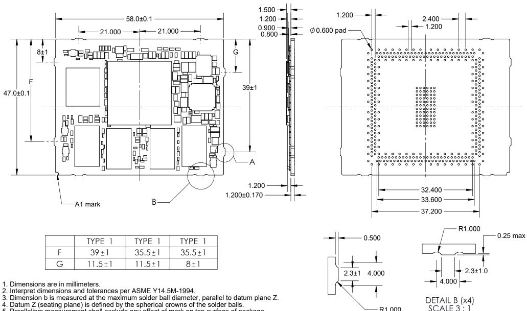
5. Parallelism measurement shall exclude any effect of mark on top surface of package.
