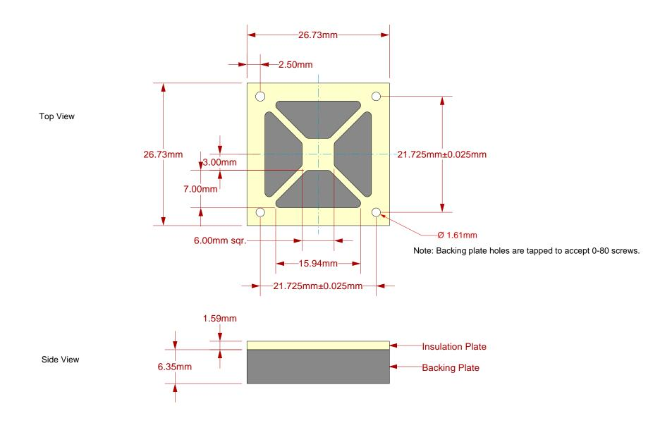
Description: Backing Plate with Insulation Plate
