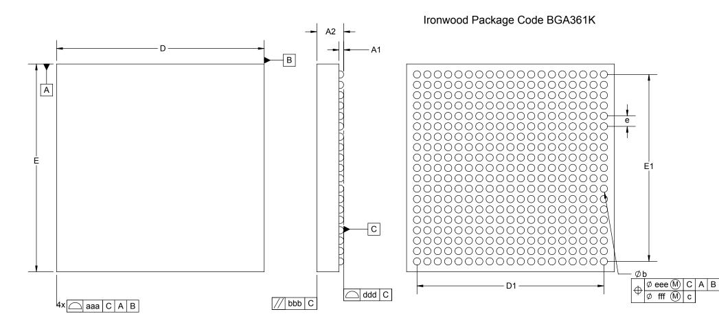
Dimensions are in millimeters.
