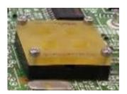
Stencils available for applying solder paste for sockets that do not have solder balls attached
