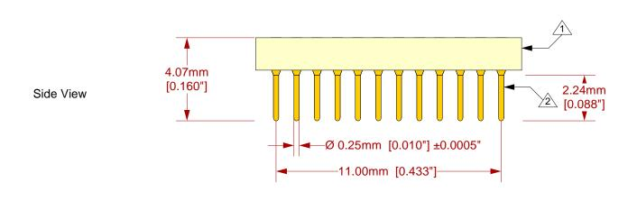
Substrate: 1.59mm ±0.18mm [0.0625" ±0.007"] T FR4/G10 or equivalent high temp material.
