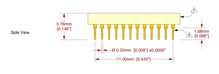
Substrate: 1.59mm ±0.18mm [0.0625" ±0.007"] FR4/G10 or equivalent high temp material.
