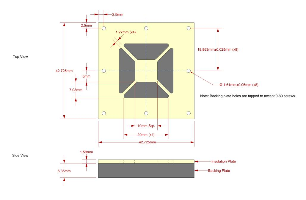
Description: Insulation Plate and Backing Plate
