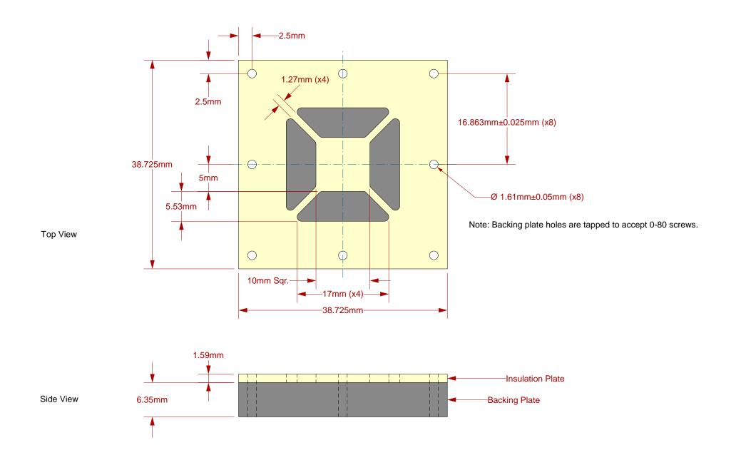
Description: Insulation Plate and Backing Plate
