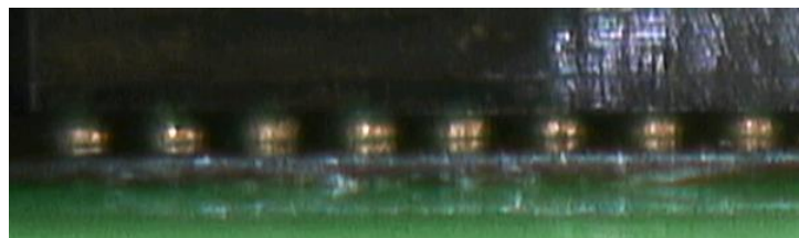
Image above shows Grypper Socket attached to PCB. Reflowed solder paste forms solder joint between Grypper Contacts and PCB pads
