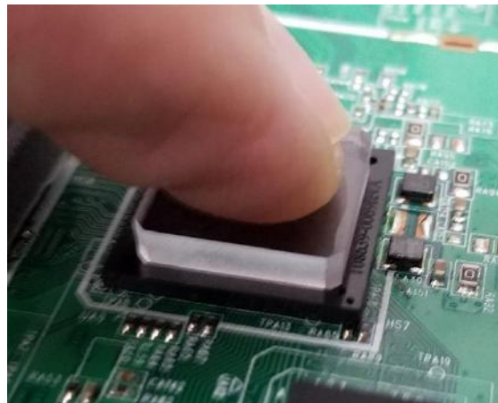
Device inserted on applications where under approximately 20 pounds or less are needed your thumb / finger can insert the device
