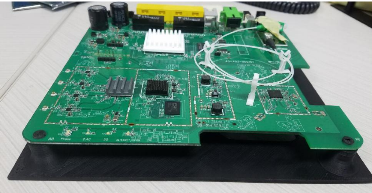
PCB placed on New Test Fixture with supports
