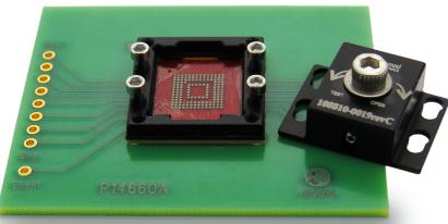
High Performance Near Zero Footprint Sockets for 0.25 + pitch devices for Both BGA and lead and leadless packages. New Configuration using the proven GT elastomeric contact element allowing 43 Ghz Bandwidth (Measured on 0.5 pitch BGA -S21 @-1dB @ 43 GHz) 1000+ insertions on the same device with many lid options.
