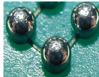
Wire marks on BGA
