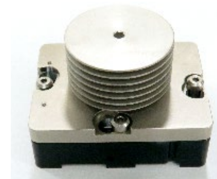
Socket with heat sink
