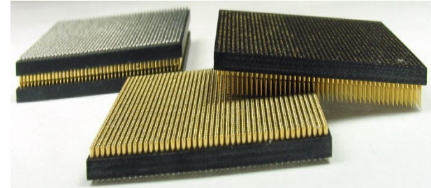
2000 pin count BGA system plugged together & shown separately
